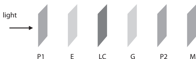
Figure 1133 The principle of a liquid crystal display (LCD)
